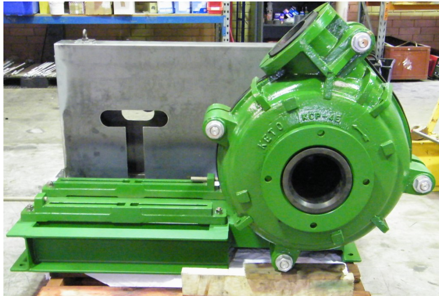
Photo 2: KETO HS-F Froth Pump – Discharge Nozzle Orientation
